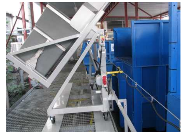
Waste cart tipper for several containers/compactors
